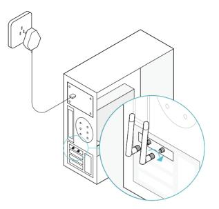
4. Replace the case panel, plug in the power cable and turn on your computer. Note:
