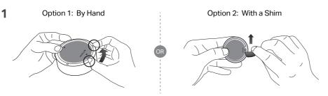
(Optional) Attach the non-slip pad to the button to keep it firmly in place. Magnetically attach the button to metallic objects.
