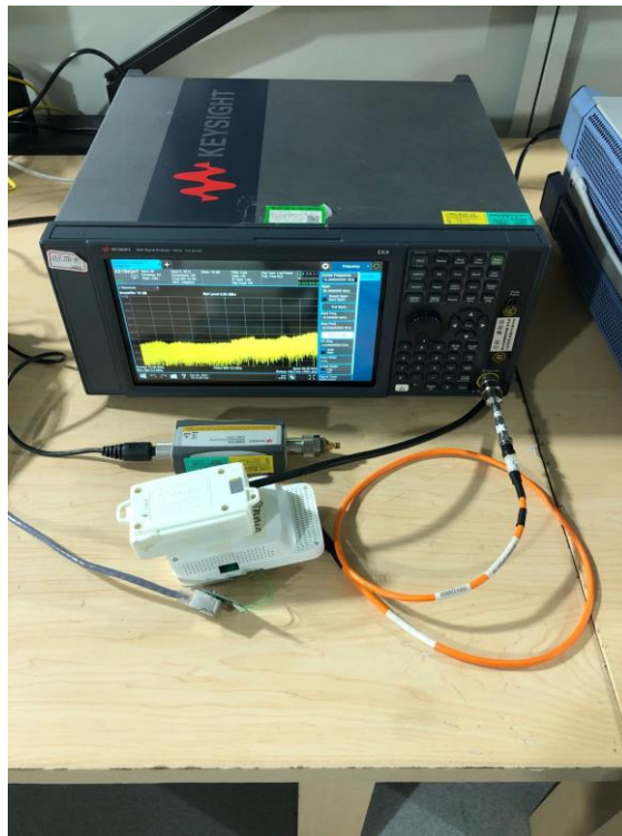
Description: Conducted Test Setup
