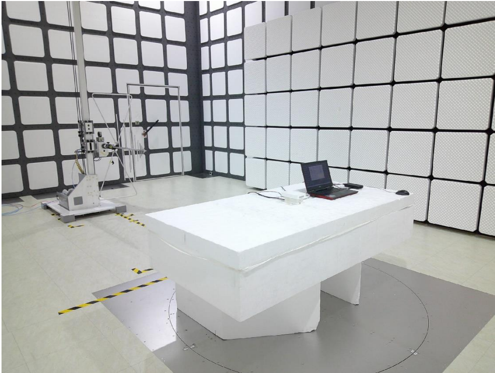
Description: Radiated Emission Test Setup for above 1GHz for WiFi
