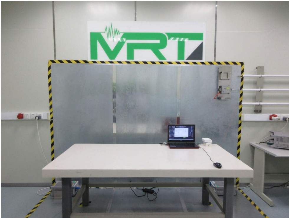
Description: Back View of Conducted Emission Test Setup for WiFi
