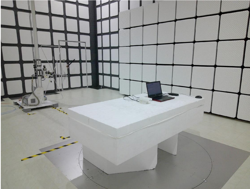
Description: Radiated Emission Test Setup for above 1GHz for BLE
