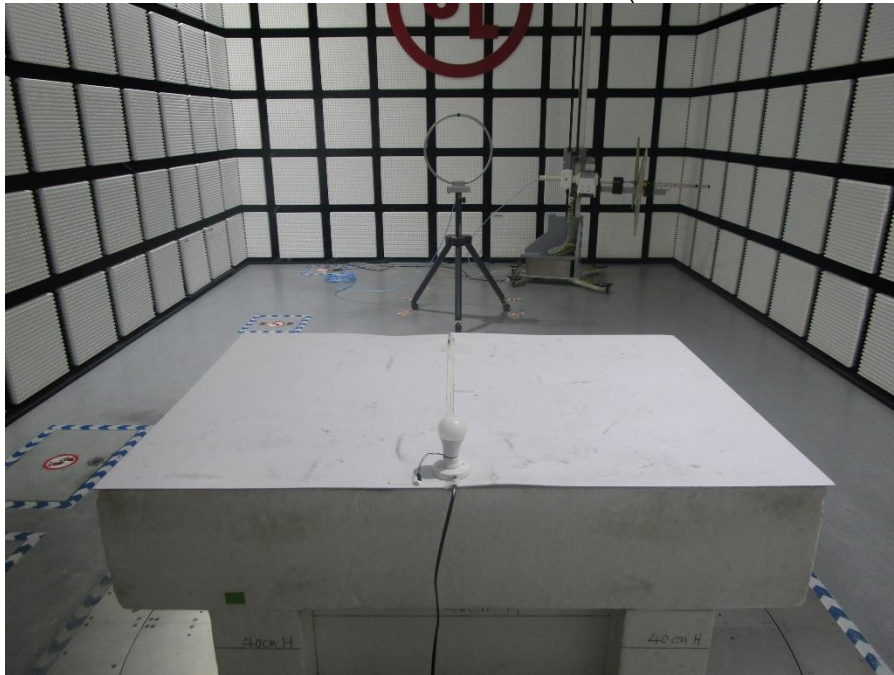
RADIATED RF MEASUREMENT SETUP (Below 30MHz)
