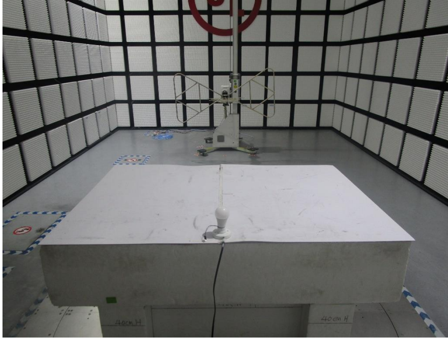
RADIATED RF MEASUREMENT SETUP (Below 30MHz)
