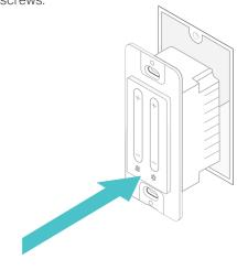
2 Ensure the UP arrow on the back of the wallplate points up and attach the wallplate. Then turn on the circuit breaker.
