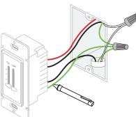
Note: DO NOT remove any wire. You might as well take a picture of the old switch wiring condition for reference.
