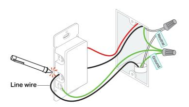
2) Turn off the circuit breaker. Check your power is off by turning your fan and light on and off a few times. Make sure your old switch is turned off before continuing wiring.
