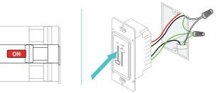
2) Use a voltage detector to identify the energized wire among the two load wires. This should be the load wire of your light switch.
