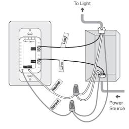
Ground: Usually green or copper. Neutral: Usually white and not connected to a dumb switch. Line: Usually black and coming from the circuit breaker. Load: Usually black. One end is connected to the light. If you are unsure, consult a qualified electrician.
