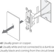
3 Identify Line and Load wires.
