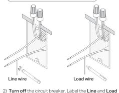
Connect the wires to the smart dimmer 4 switch as shown below.
