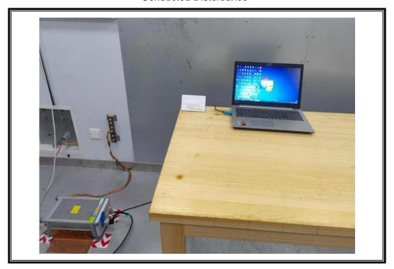
RADIATED RF MEASUREMENT SETUP (30MHz  $\sim$  1 GHz)
