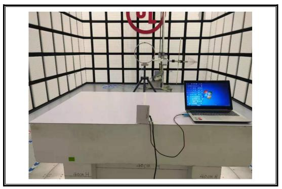
RADIATED RF MEASUREMENT SETUP (Above 1G )
