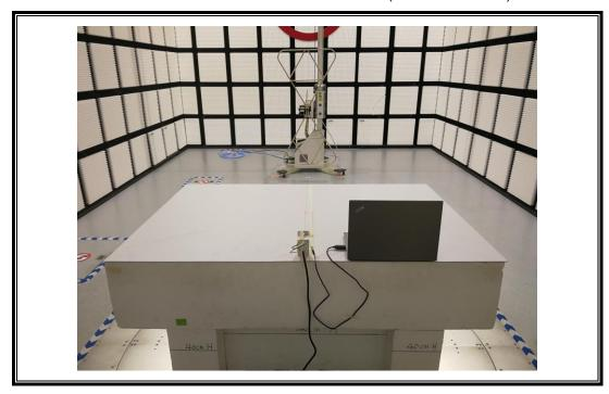
RADIATED RF MEASUREMENT SETUP (Below 30MHz)
