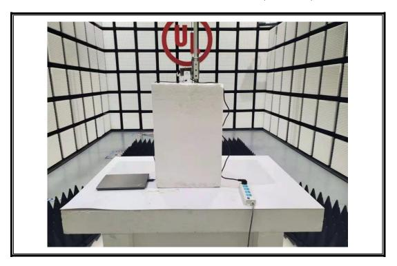
CONDUCTED RF MEASUREMENT SETUP
