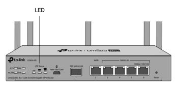
• **Reset:** Press and hold the button for 5 seconds, the SYS LED will flash quickly, indicating the device is being reset to its factory default settings.
