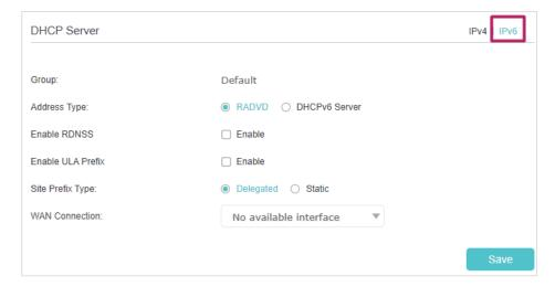
1) Select RADVD as the address type to make the router assign IPv6 address prefixes to hosts.
