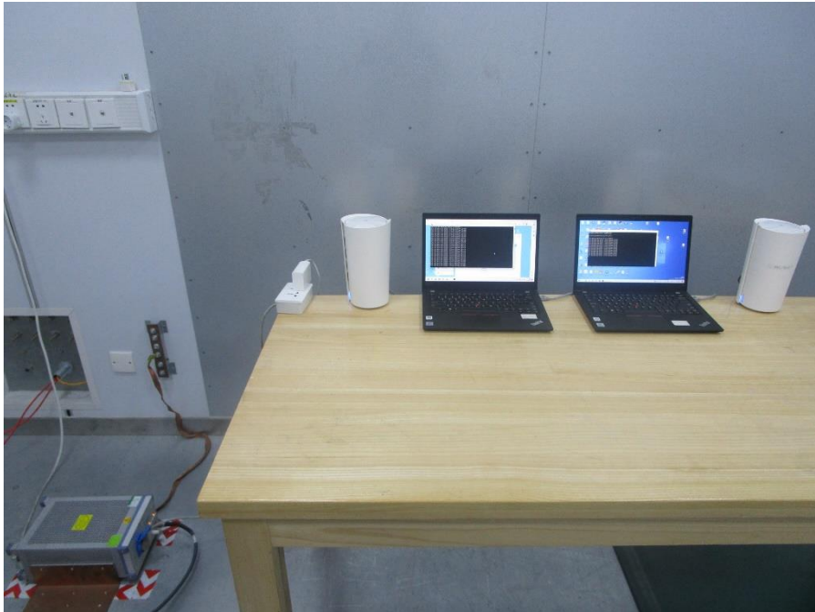
POWERLINE CONDUCTED EMISSIONS MEASUREMENT SETUP
