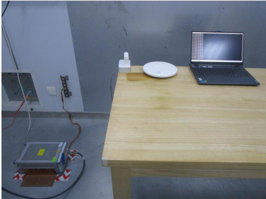
POWERLINE CONDUCTED EMISSIONS MEASUREMENT SETUP
