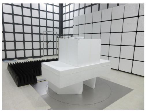
Description: Radiated Emission Test Setup for - 18GHz ~ 40GHz
