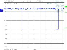
Duty cycle = 5.440 ms / 5.860 ms = 92.83% Duty Factor = 10 log(1 / Duty cycle) = 0.32
