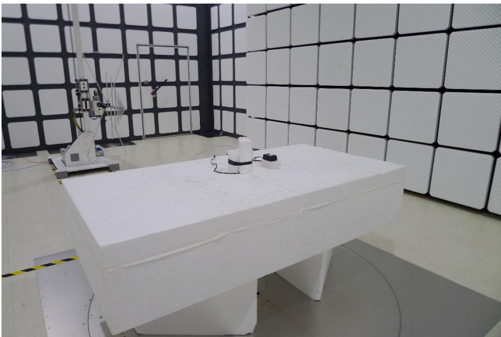
Description: Radiated Emission Test Setup for 30MHz ~1GHz
