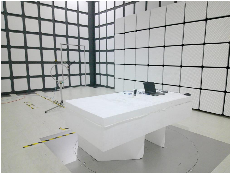
Description: Radiated Emission Test Setup for 9kHz~30MHz
