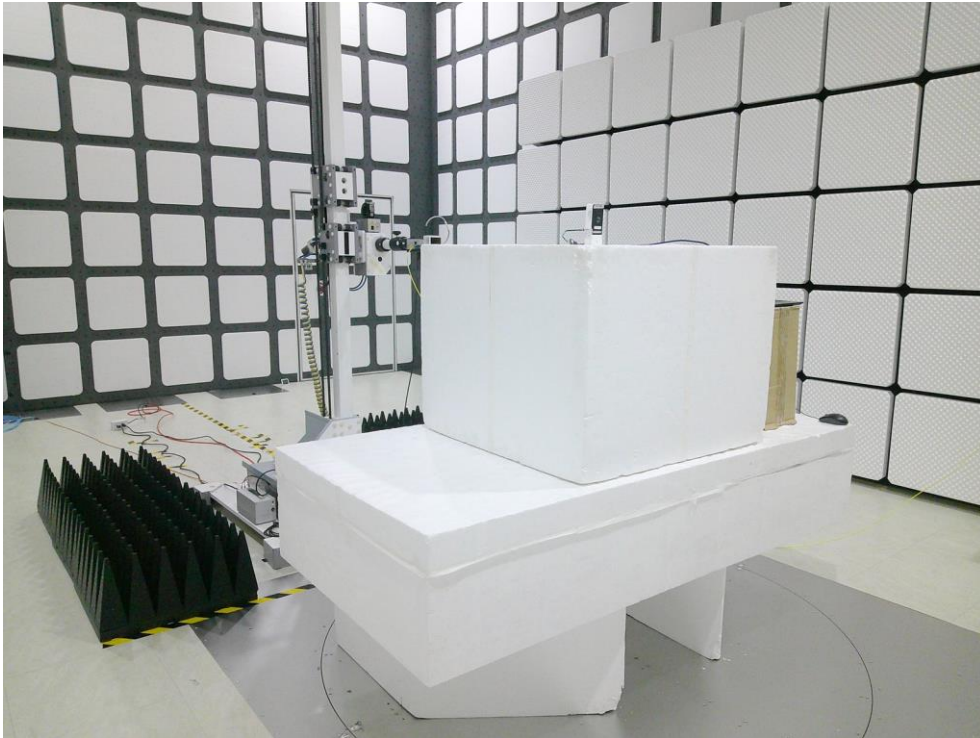
Description: Radiated Emission Test Setup for 9kHz~30MHz
