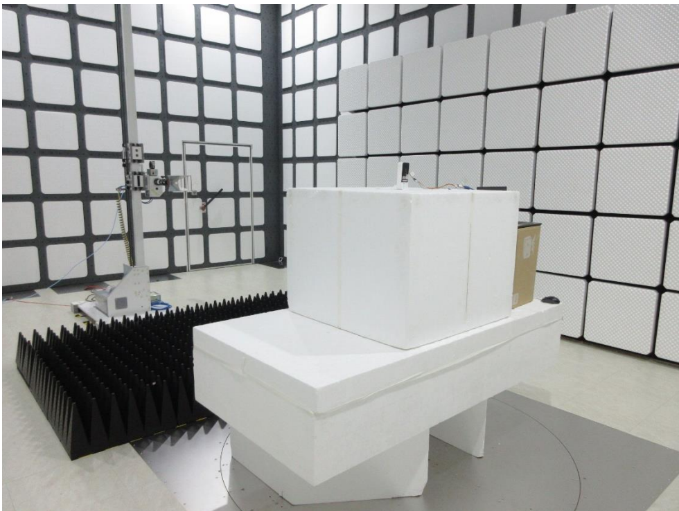
Description: Radiated Emission Test Setup for 1GHz~18GHz
