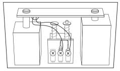
4. Tighten the screws and replace the chime cover.
