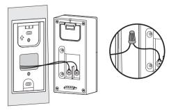
Mount the doorbell to the bracket and turn on the circuit breaker.
