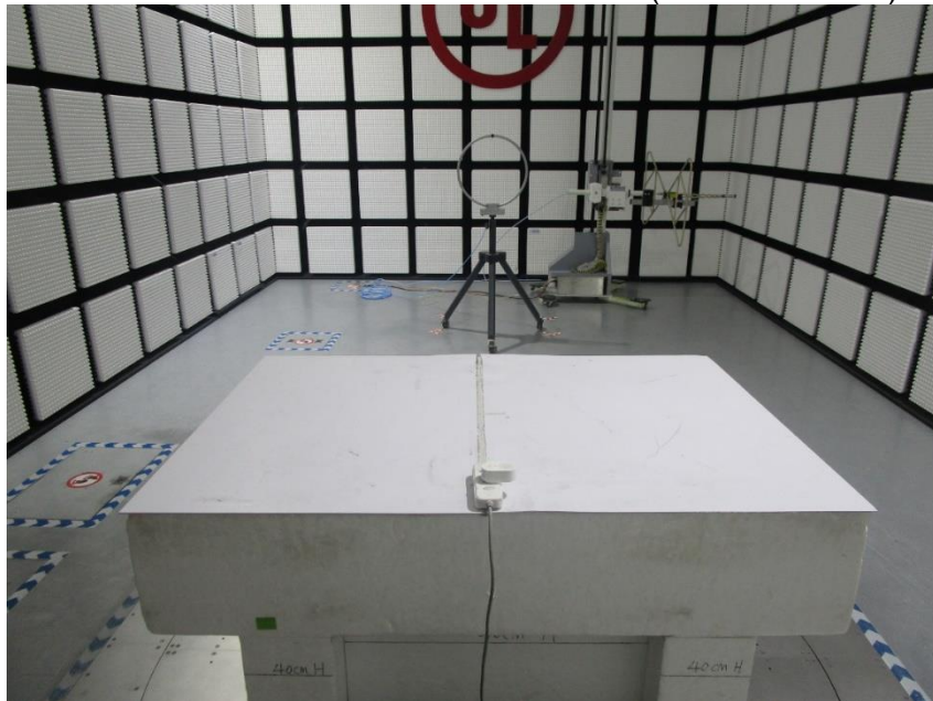
RADIATED RF MEASUREMENT SETUP (BELOW 30MHz)
