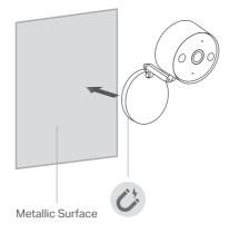
This equipment shall be installed at a height of fewer than 2 meters.
