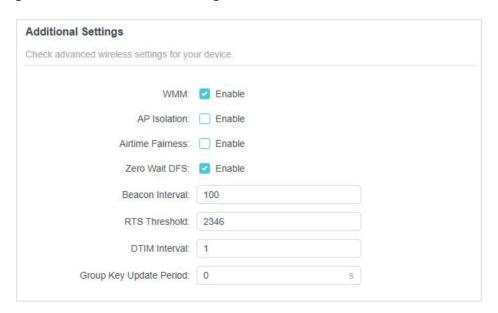
WMM - WMM function can guarantee the packets with high-priority messages being transmitted preferentially.
