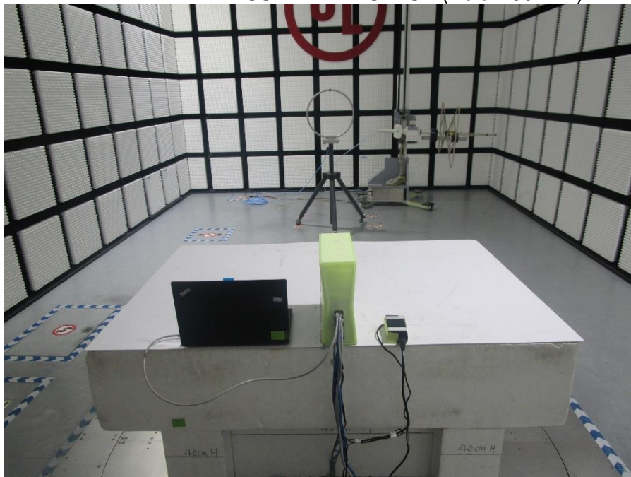
RADIATED RF MEASUREMENT SETUP (Below 30MHz)
