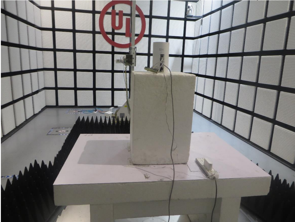
RADIATED RF MEASUREMENT SETUP (30 MHz ~ 1 GHz)
