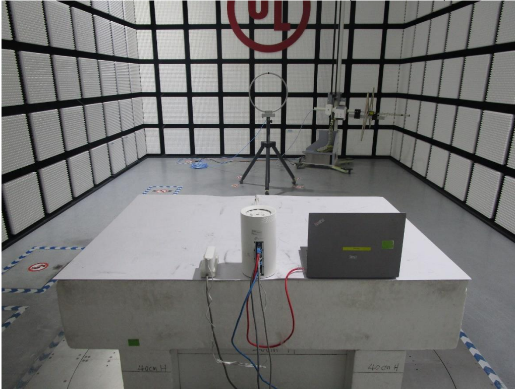
POWERLINE CONDUCTED EMISSIONS MEASUREMENT SETUP
