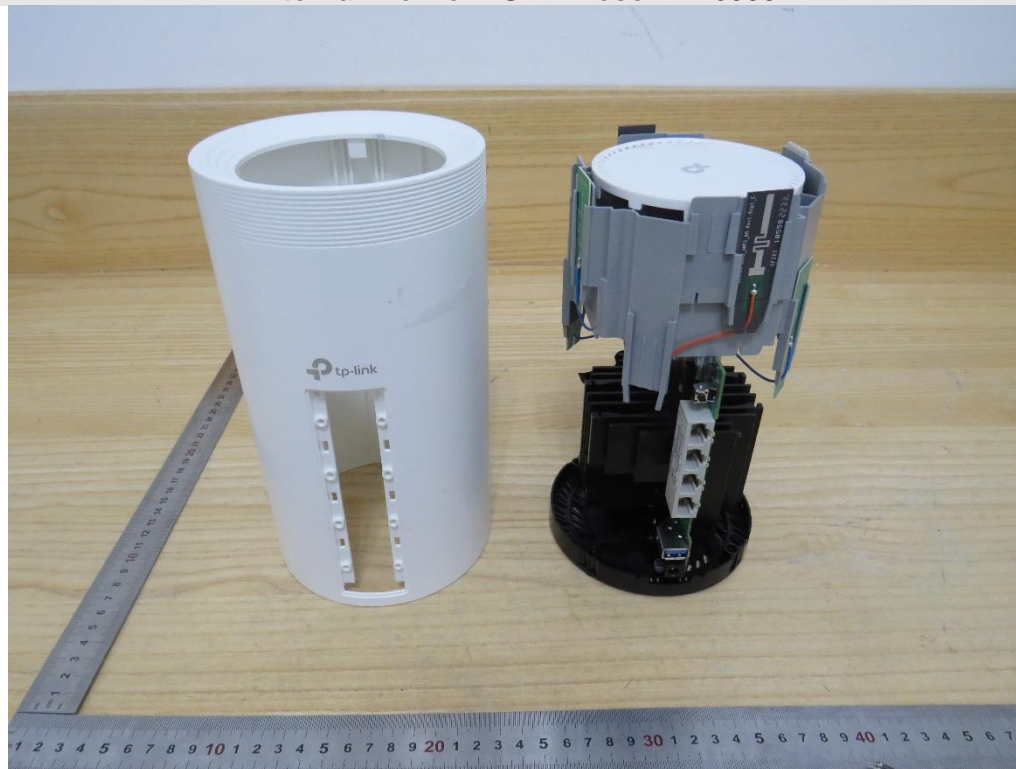
Internal View of EUT-1-Deco BE16000
