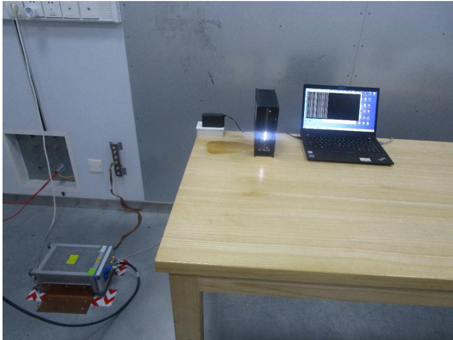
POWERLINE CONDUCTED EMISSIONS MEASUREMENT SETUP
