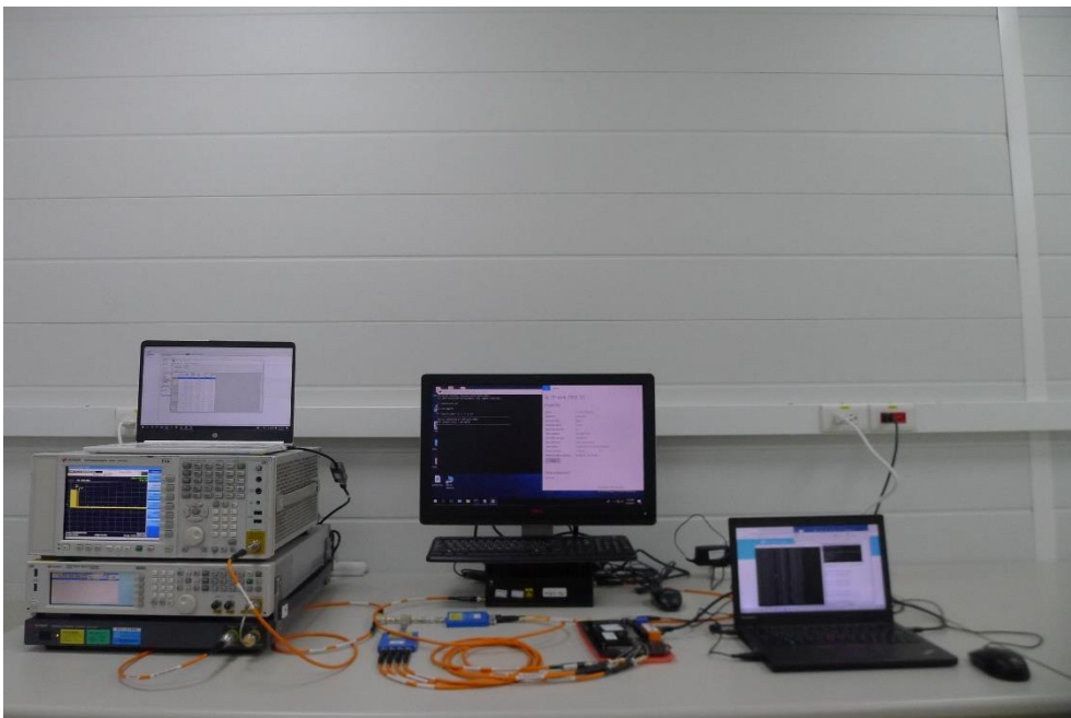
Description: DFS Test Setup
