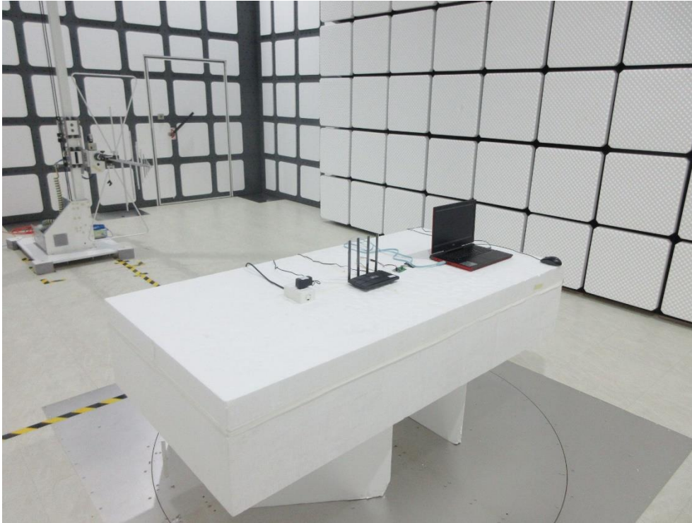
Description: Radiated Emission Test Setup for 1GHz~18GHz
