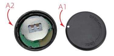
②Align position A1 with A2, then clockwise rotation to lock.
