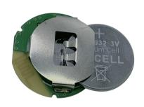
①Put the battery into card slot. Pay attention to the battery direction: Positive pole upward.
