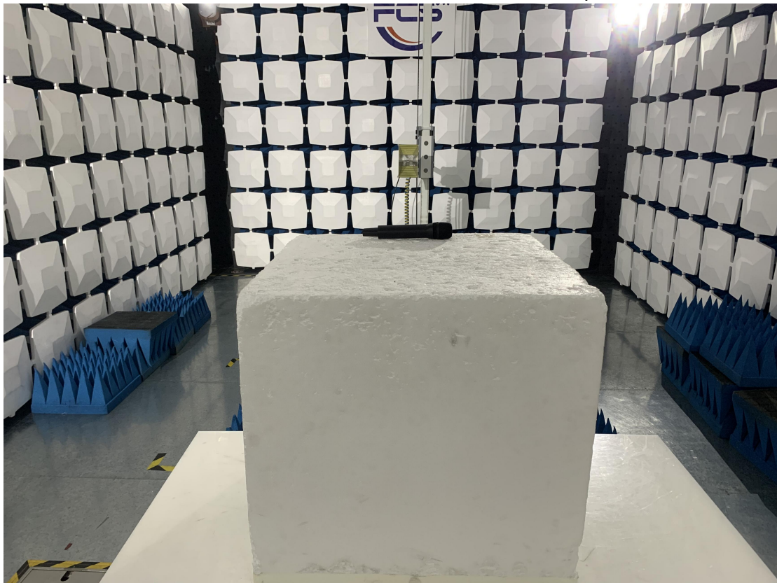
Above 1GHz for radiated emission test setup
