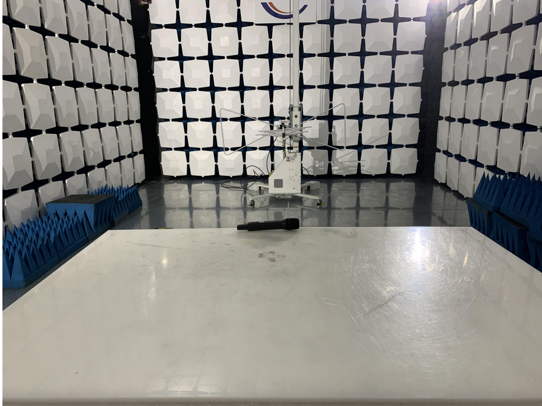
Above 1GHz for radiated emission test setup
