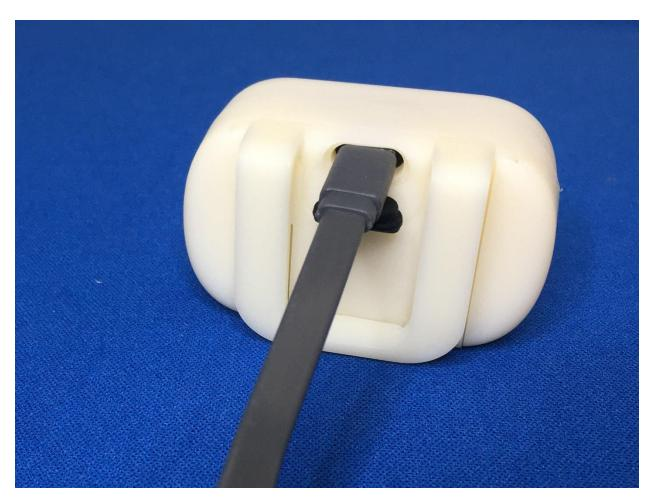
Figure 3 Link 3 - Back showing cable inserted in charging port through clip.
