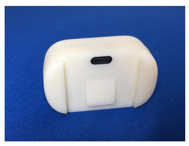
Figure 2 Link 3 - Back showing charging port without clip.
