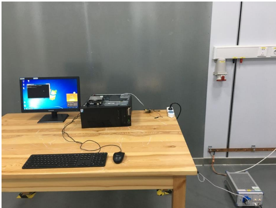
Fig. 4 Power line conducted emission setup photo
