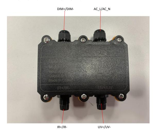
The input and output pins of the product are shown in the figure. Install the product into the LED lamp, connect the corresponding dimmer and special infrared and ultraviolet lamps, and then connect and use through APP. The product has two Bluetooth modules, which can be networked and can be realized on the APP.
