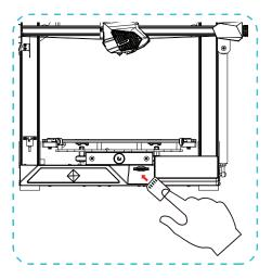
6.Insert the storage card→ Click print control→ Select the file to be printed. 插入存储卡→点击打印控件→选择 要打印的文件
