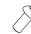
10 M5x12 Hexagon flat round head screw x2 M5x12内六角平圆头螺丝
