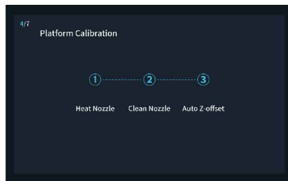
8. For platform calibration, complete nozzle heating, nozzle cleaning and nozzle alignment sequentially.
