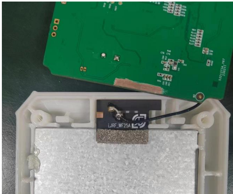
Chart 3 Add conductive foam to connect with PCB
