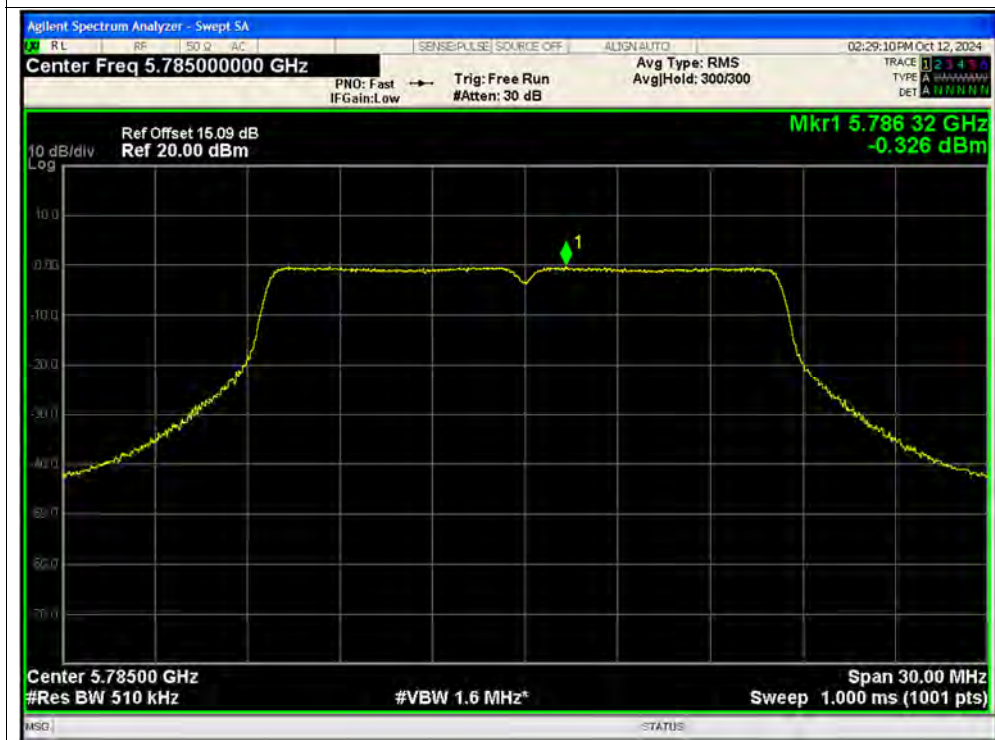
PSD NVNT a 5825MHz Ant2 SISO
