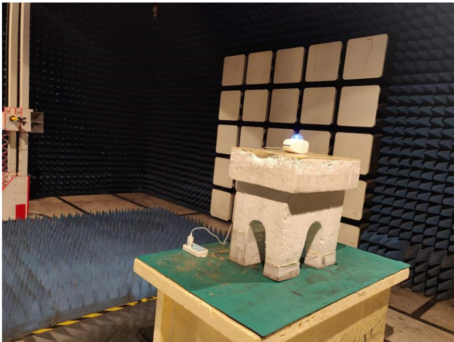
Spurious Emission Test Setup (Above 1GHz)
