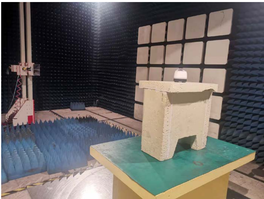
Spurious Emission Test Setup (Above 1GHz)
