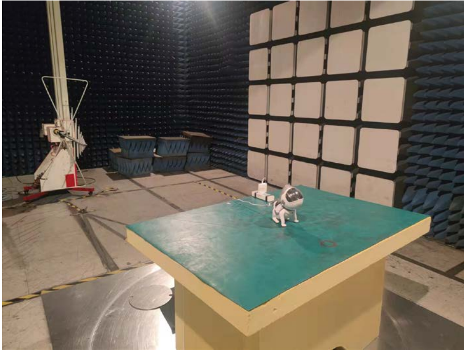
Spurious Emission Test Setup (Below 1GHz)
