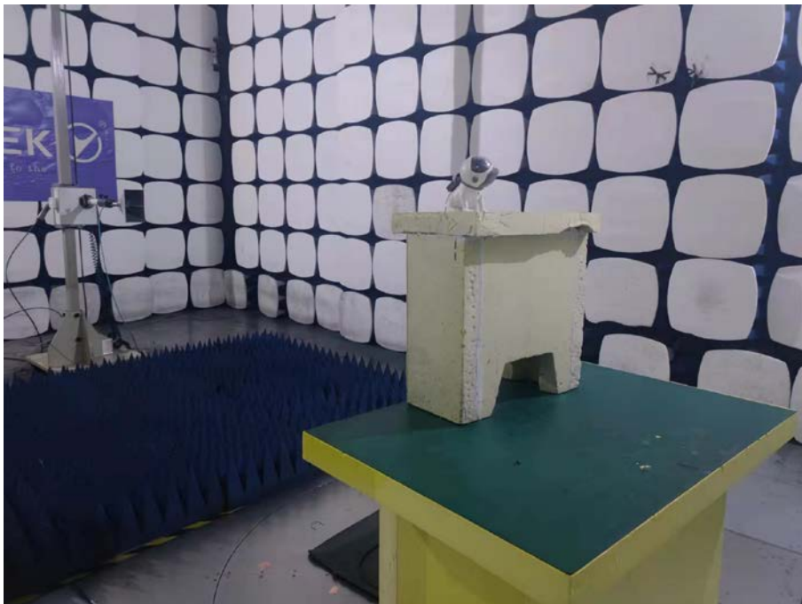
Spurious Emission Test Setup (Above 1GHz)
