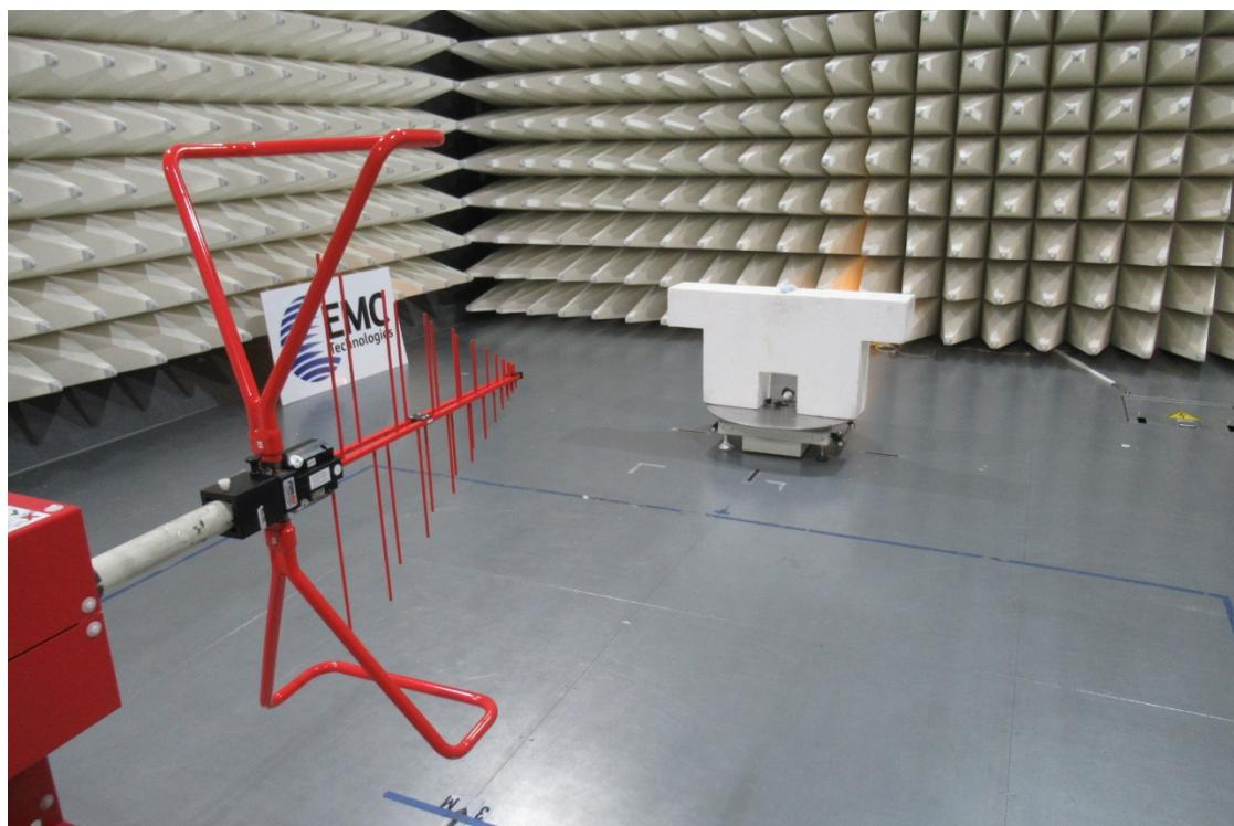
Radiated Emissions: 30 MHz to 1000 MHz
