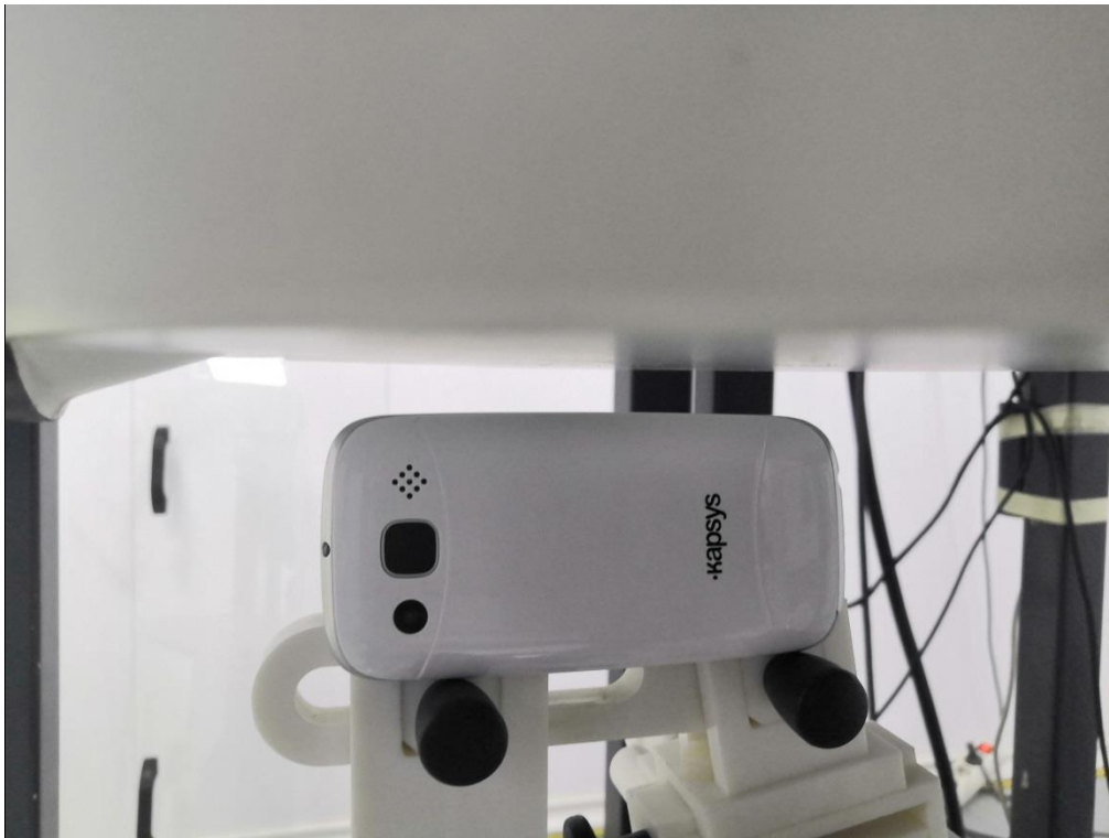
10mm body-worn Left Side Setup Photo (hotspot)
