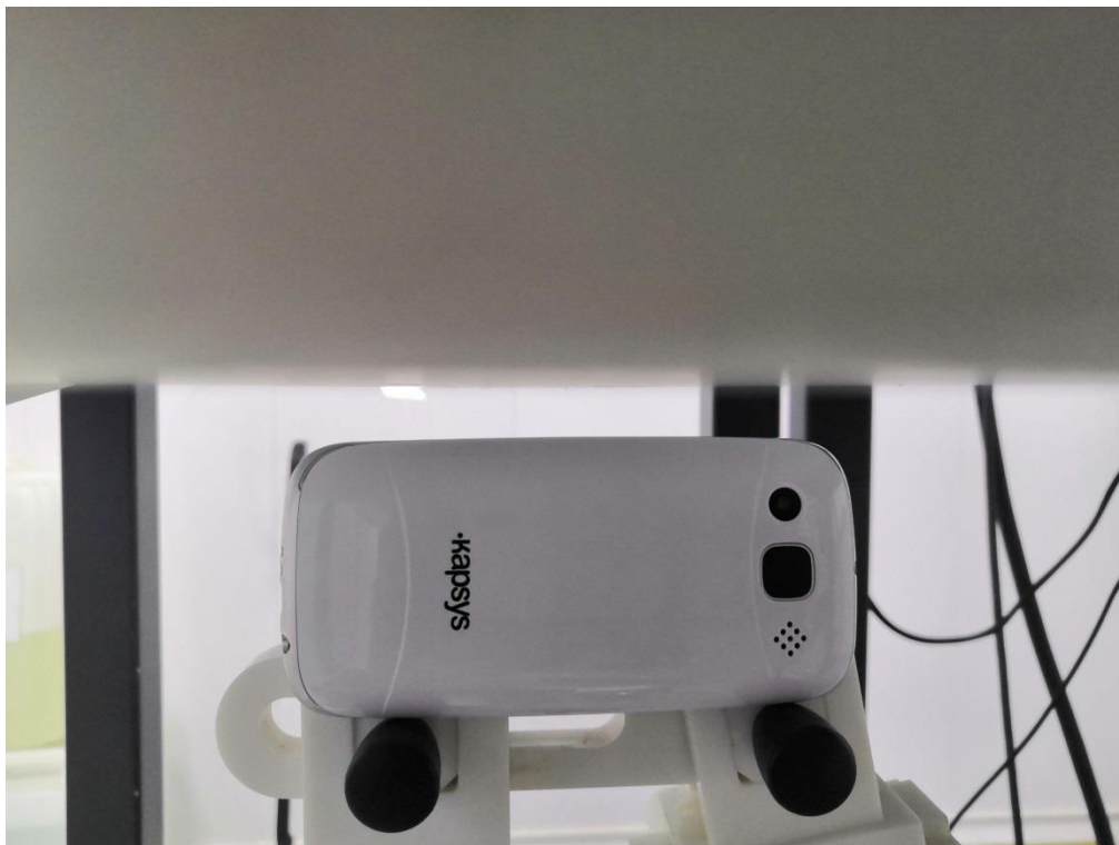
10mm body-worn Right Side Setup Photo (hotspot)
