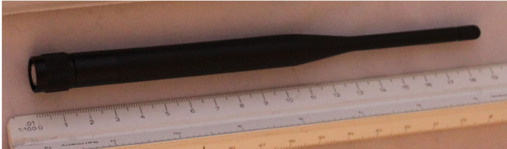
Nearson S151TC-2450 non-articulated TNC-Male connector Gain 5dBi VSWR 2:1 Vermeer Part Number: 296575379
