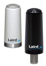
Laird Connectivity's unique Phantom® antenna operates simultaneously in the 698-960 MHz and 1700-2700 MHz bands, making it ideal for 4G/3G applications where no ground plane or metal surface is available. The mechanically robust design is suitable for both indoor and outdoor applications with wide bandwidth and a low angle radiation pattern that is superior to traditional gain antennas in most applications. The antenna is ideal for both ceiling and surface mount applications.
