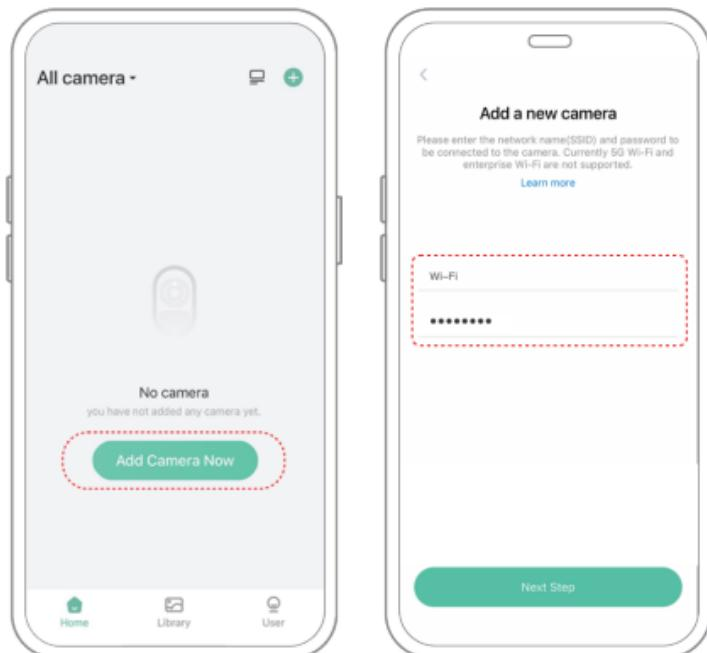
2) To ensure a longer distance connection, the camera only supports the 2.4Ghz Wi-Fi with stronger wall penetration capability and does not support Wi-Fi for enterprise level authentication currently. Please ensure that the entered Wi-Fi meets the requirements. After completion, click "Continue" to generate the QR code for pairing the camera.
