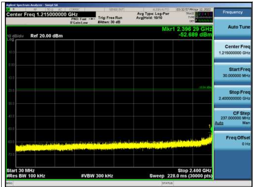
Test_Graph_802.11g_ANT1_2437_6Mbps_Lower Band Emissions
