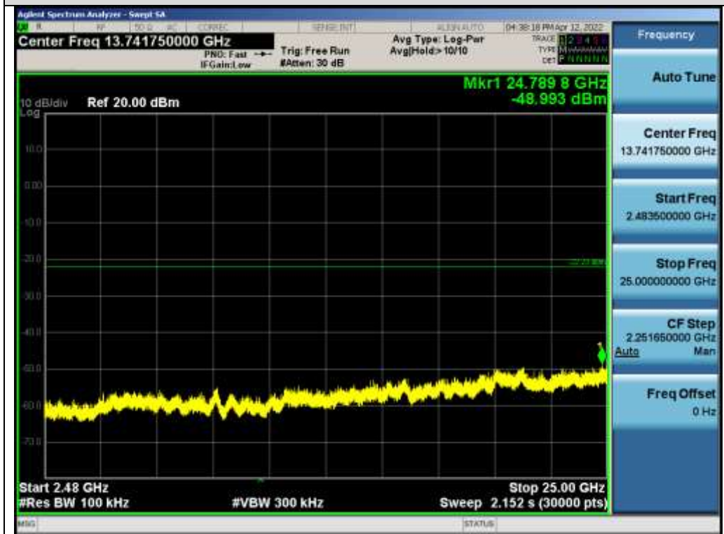
Test_Graph_802.11n20_ANT1_2412_MCS0_Higher Band Emissions
