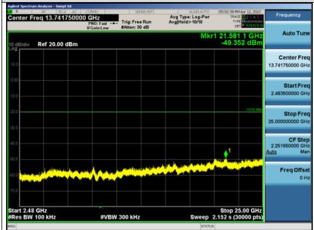
Test_Graph_802.11g_ANT1_2412_6Mbps_Higher Band Emissions
