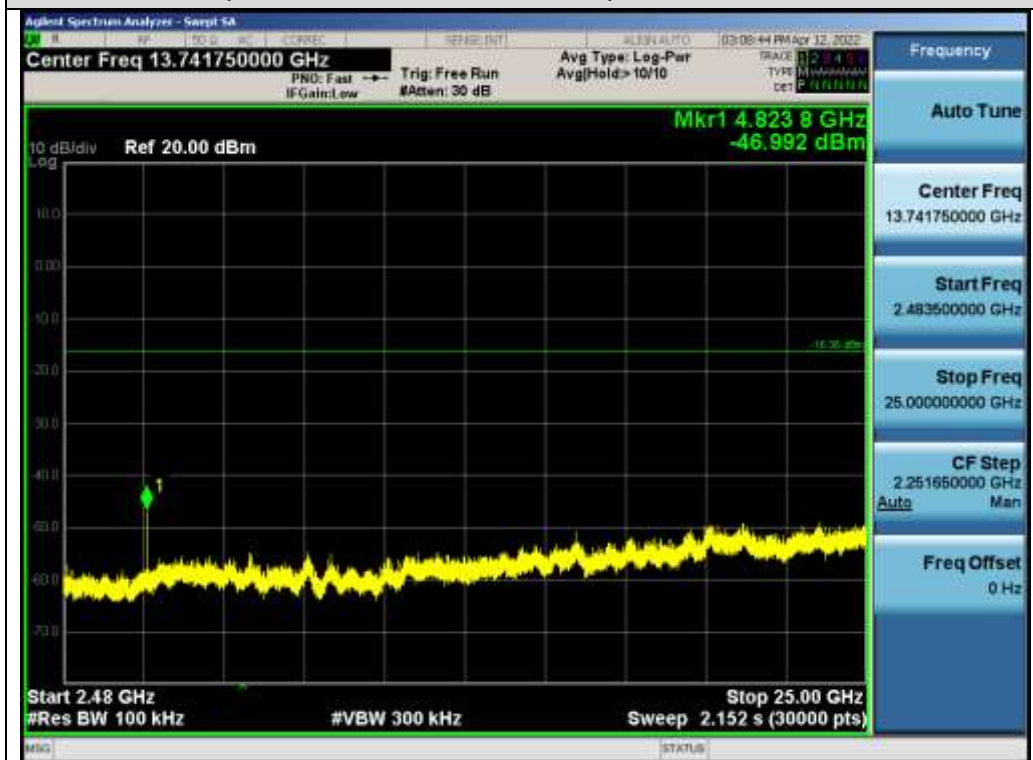
Test_Graph_802.11b_ANT1_2412_1Mbps_Higher Band Emissions
