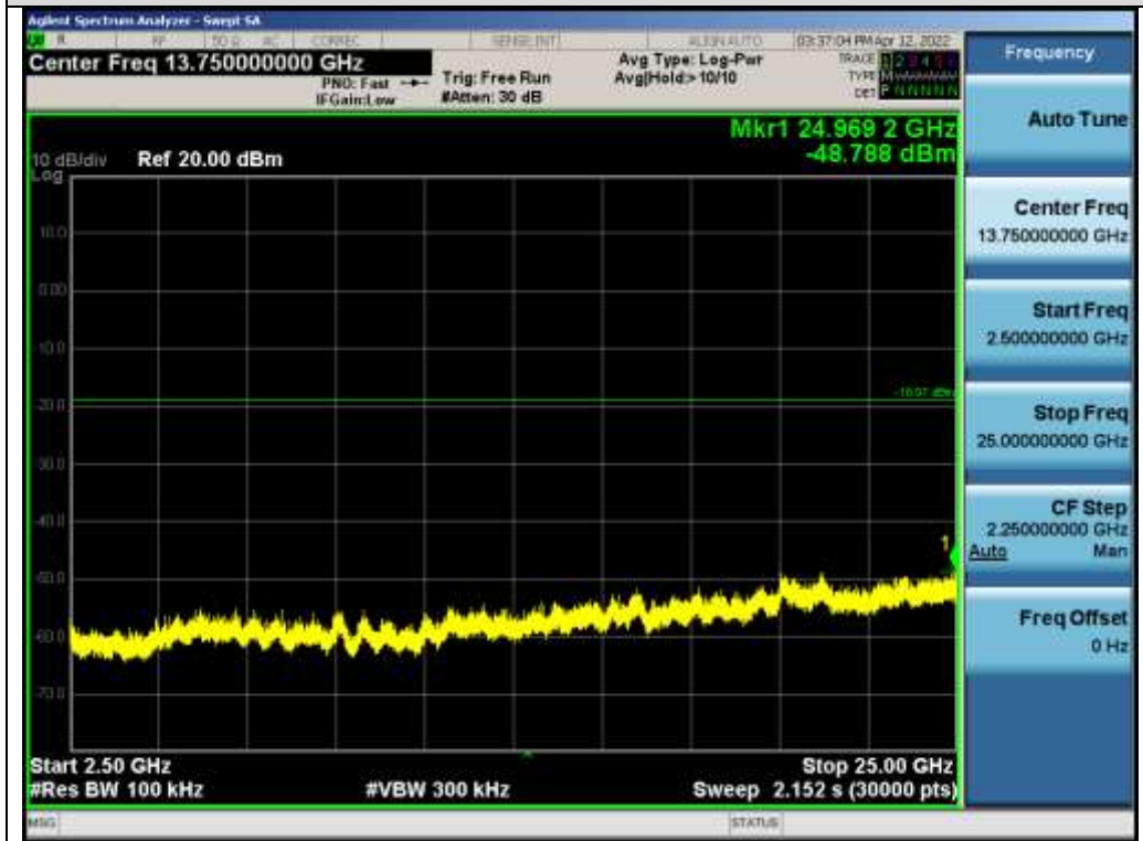
Test_Graph_802.11g_ANT1_2462_6Mbps_Higher Band Emissions
