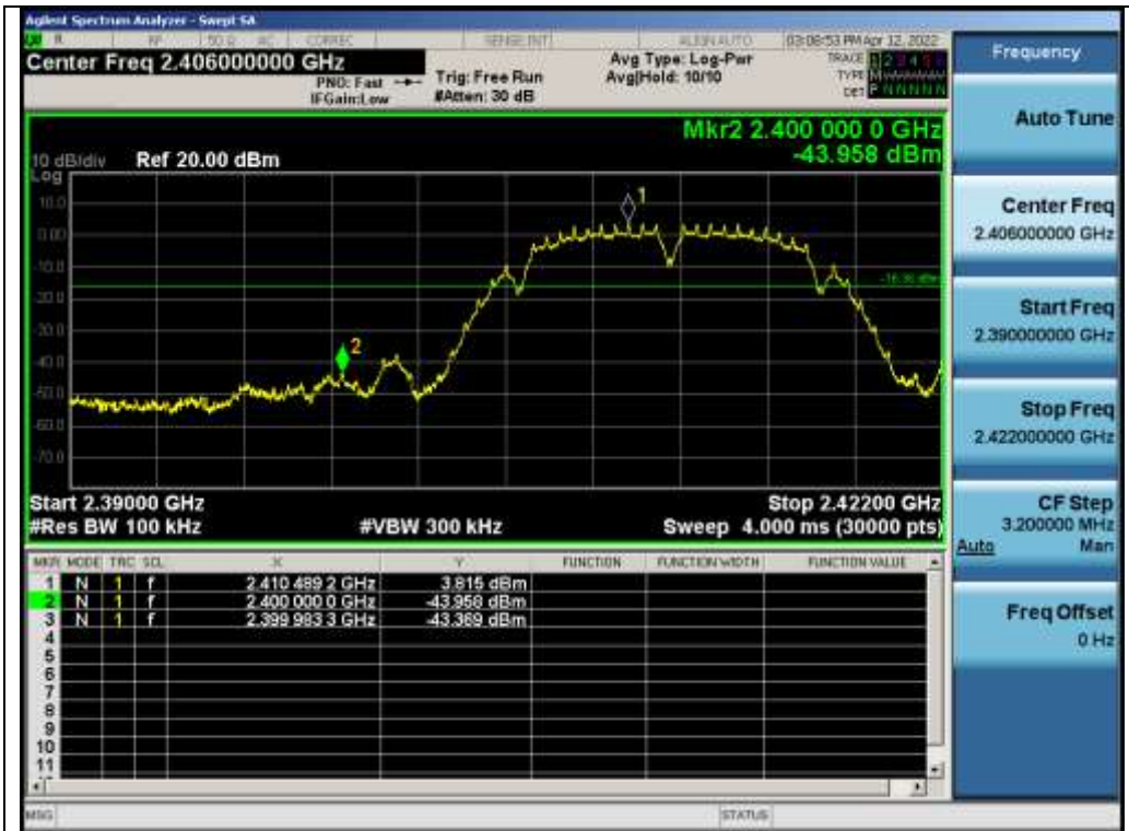
Test_Graph_802.11b_ANT1_2412_1Mbps_Lower Band Edge Emissions
