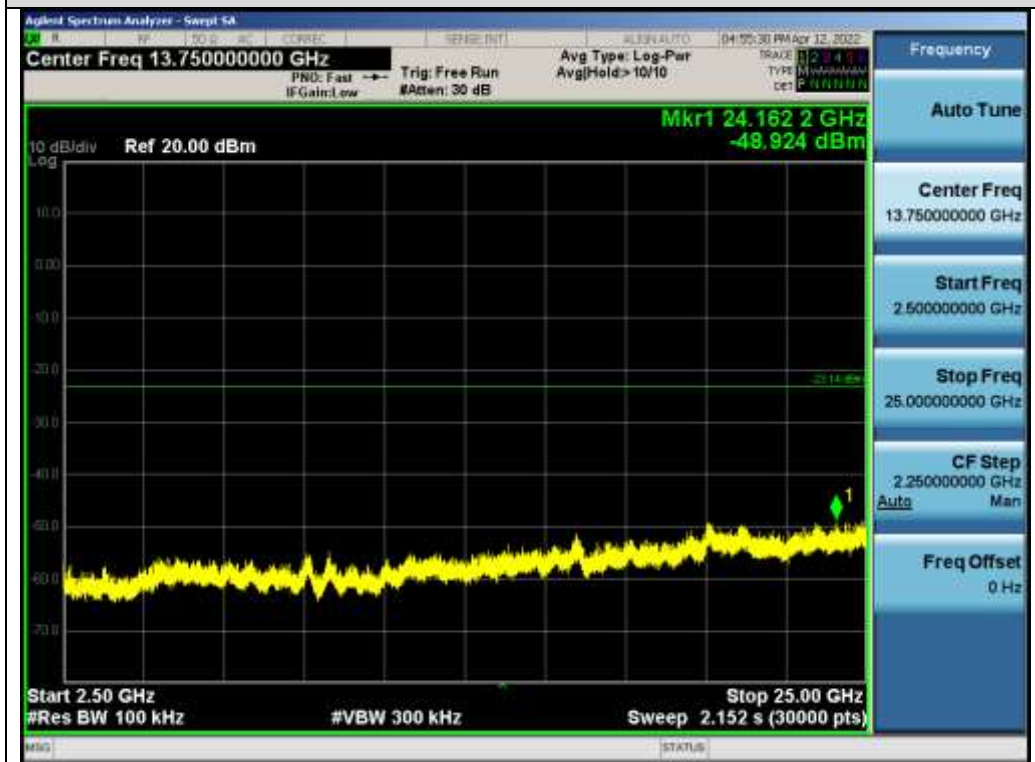
Test_Graph_802.11n20_ANT1_2462_MCS0_Higher Band Emissions
