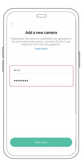
To ensure a longer distance connection, the camera only supports the 2.4Ghz Wi-Fi with stronger wall penetration capability and does not support Wi-Fi for enterprise level authentication currently. Please ensure that the entered Wi-Fi meets the requirements. After completion, click "Continue" to generate the QR code for pairing the camera.
