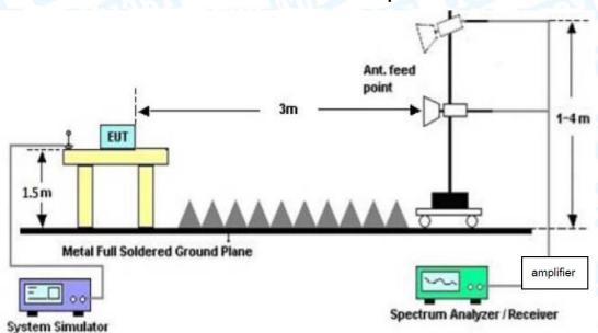
**Above 1GHz Test Setup**
