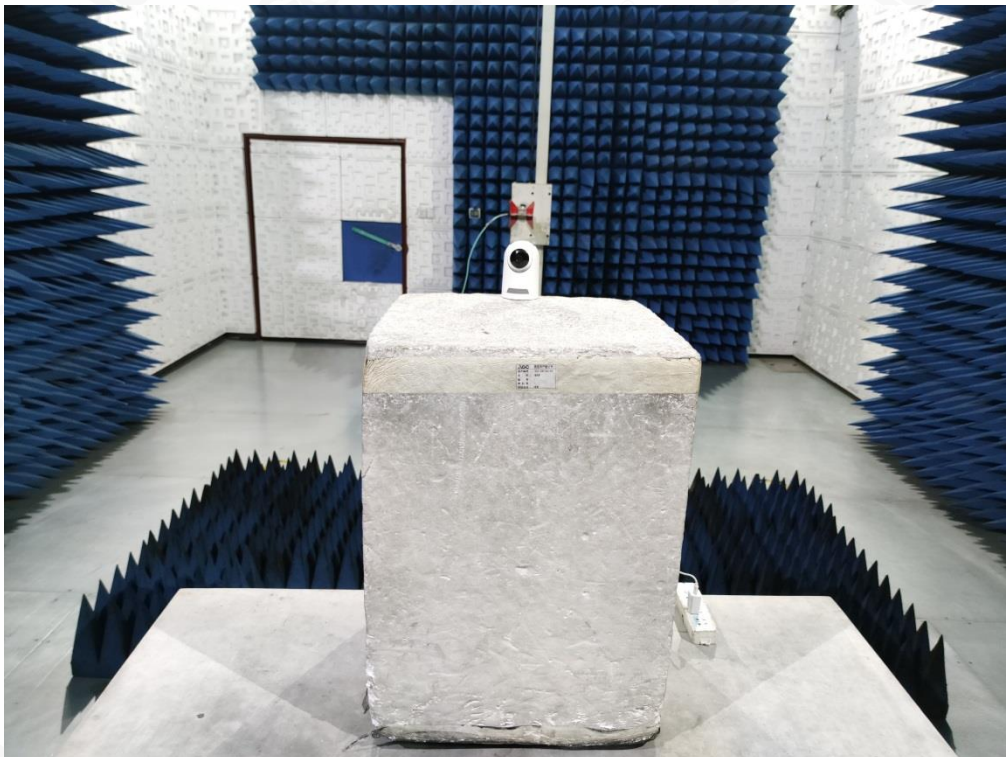
FCC RADIATED EMISSION TEST SETUP ABOVE 1GHZ
